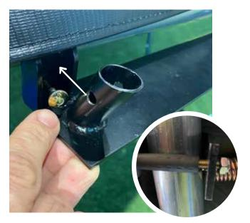
Attach the **base plate** to the top rail, using **2 large bolts, 2 rubber spacers, 2 washers** and **2 nuts**. Thread the bolt through so that the nut is attached on the spring-side end.
